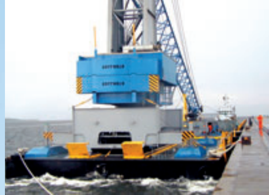
Crane transport by pontoon via a short sea route in quiet waters
