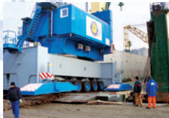
Moving the crane onto a RoRo ship
