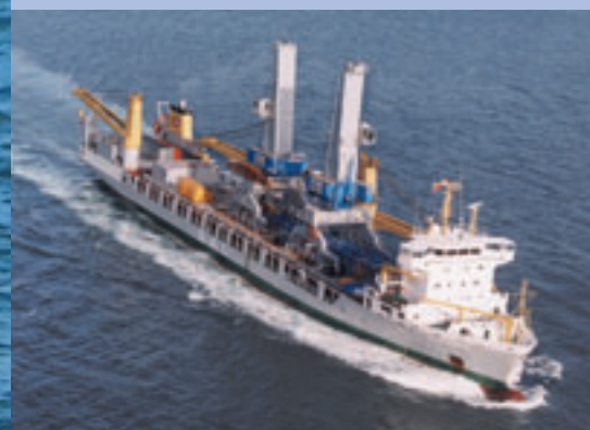
Transport of two completely assembled Gottwald cranes using a heavy-load carrier
