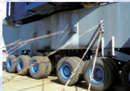
Gottwald crane secured to ensure the highest degree of stability and safety during transport
