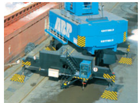
HMK 260 EG in Immingham, UK: the field-tested H-shaped stabiliser arrangement enables the crane to operate even in areas with a minimum of working space
