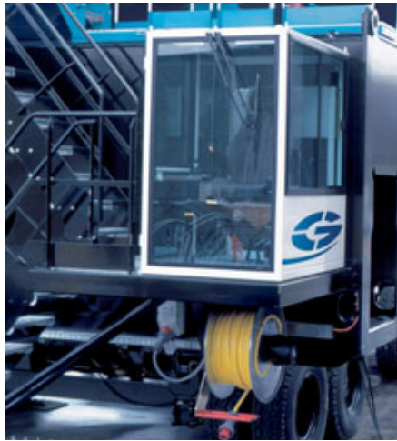
Additional cab on the chassis
