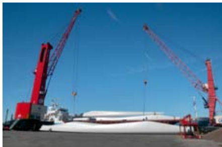
Outsized cargo require tandem lifts
