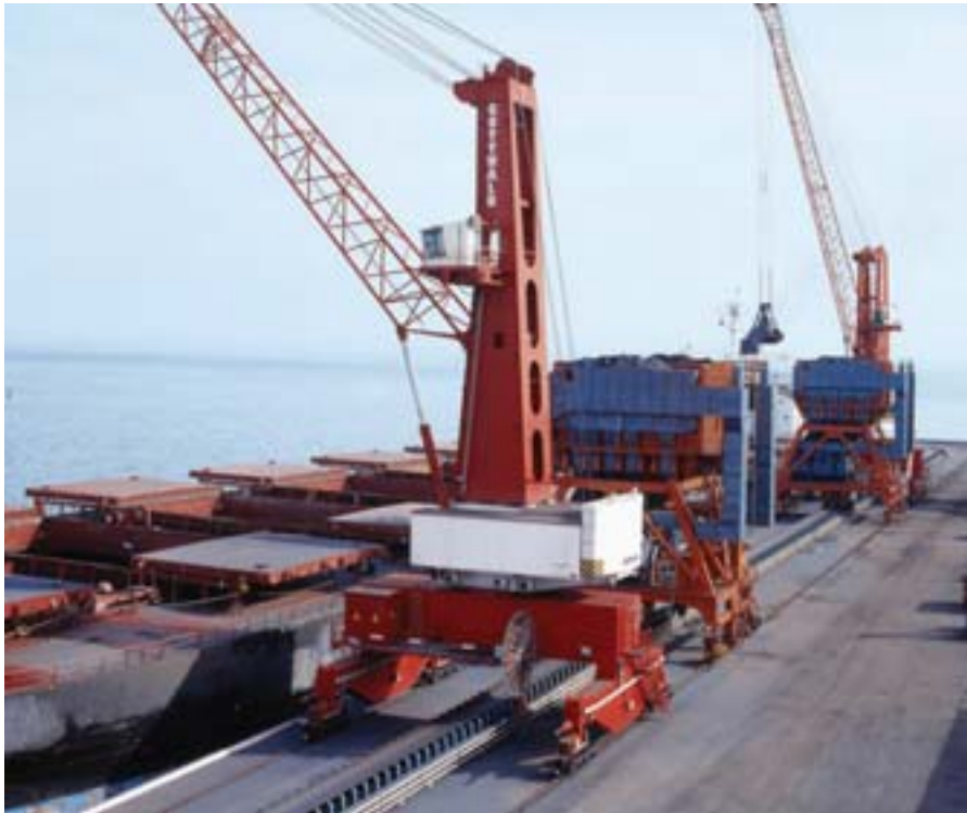
The iron ore terminal at Quinhuangdao in China has two Gottwald HSK 360 EGs.
