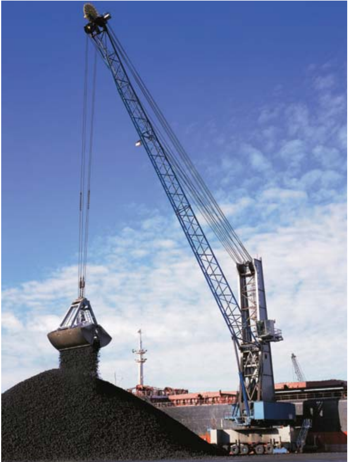
Gottwald's HMK 330 EG handles a broad spectrum of bulk materials, including fertilizers, minerals and grain. Peak loads of 1,000tph have been reached.
