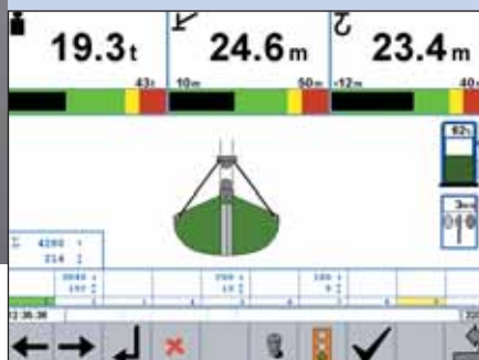
Recording the bulk handled in terms of lifts and tonnage per ship hold
