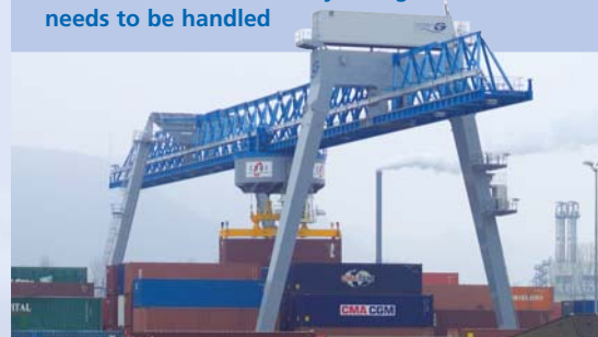
Thanks to the remote control system, the time-consuming climb to the cab of a WSG can be avoided when only a single container needs to be handled
