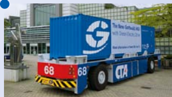
Gottwald launches the first AGV to have a diesel-electric drive
