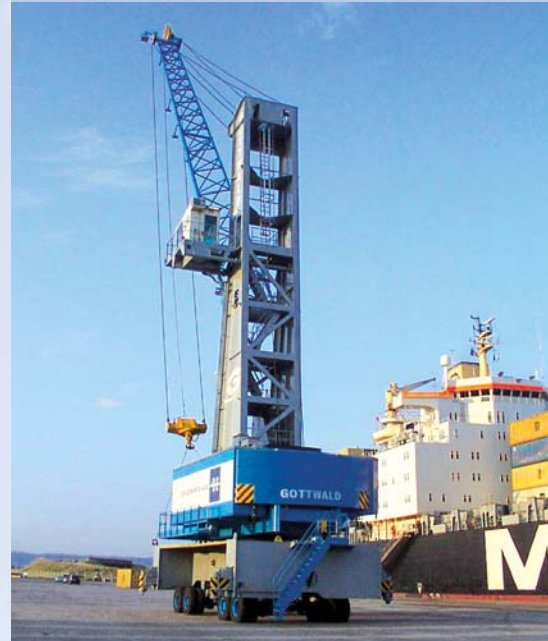
Repositioning an HMK 170 E by means of the Gottwald remote control system over a distance of 4 km at Port Autonome du Havre, France
