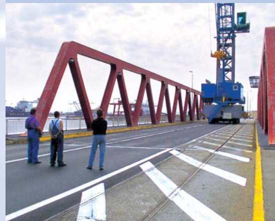
Repositioning an HMK 170 E by means of the Gottwald remote control system over a distance of 4 km at Port Autonome du Havre, France
