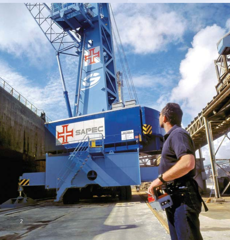
Travelling and controlling an HMK 170 EG via Gottwald's remote control system on a very narrow quay at Sapec, Portugal
