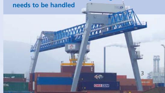
Thanks to the remote control system, the time-consuming climb to the cab of a WSG can be avoided when only a single container needs to be handled
