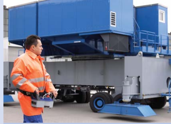
Using the remote control system at ground level, the crane operator can move the crane carefully and position it accurately
